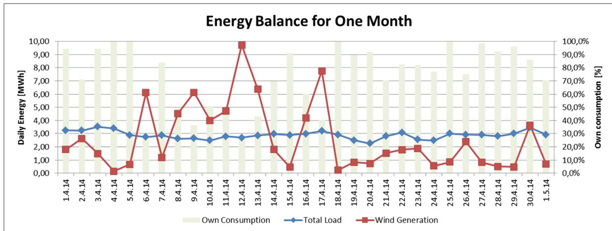
Figure 11: Self consumption, total load and wind generation for April 2014. Values represent daily energy balances calculated from quarter-hourly measuring parameters.
