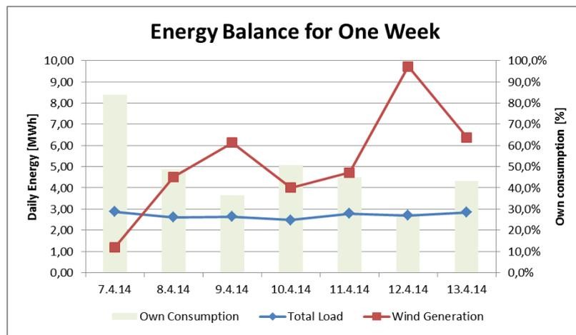
Figure 15: Self-consumption, total load and wind generation for one week starting 07 April 2014 without optimization.
