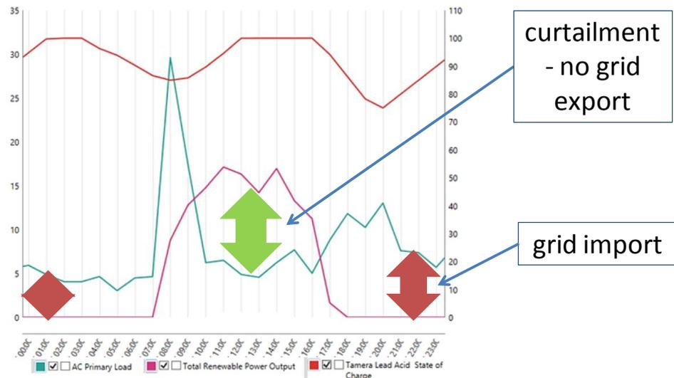
Figure 7: Current electrical situation at Tamera and Tamera PV system.
