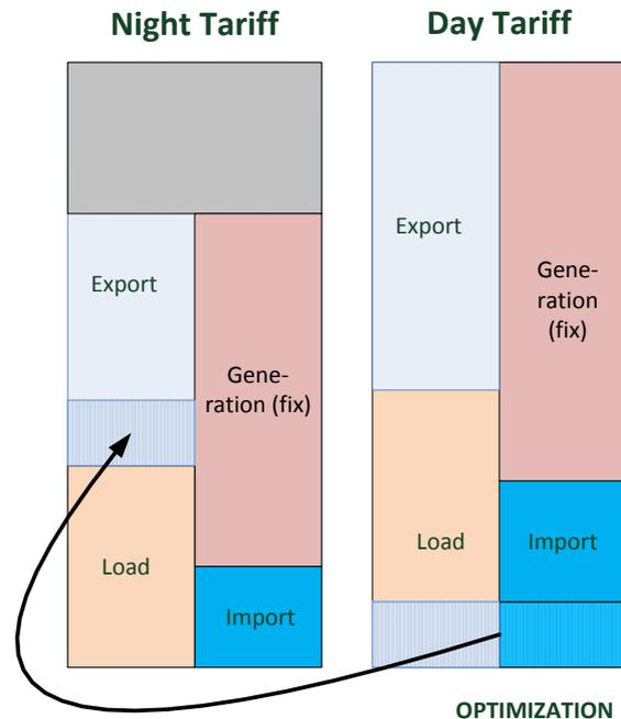
Figure 13 illustrates the options and approach for the optimisation of the energy management. There are three variables for optimization: export, import and load. The current investigation presumes that there is only one sort of electrical generator involved: wind turbines. Thus the generation at a certain time is a given value that could not be changed by the optimizer. The theoretical option of intentional lowering of the wind turbines' output has no actual meaning in the given context.
