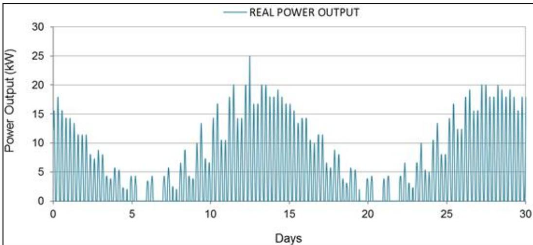
Figure 6: Tidal flow generation device power output.
