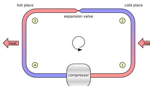
Figure: Scheme of working principal for heat pumps (source: Wikimedia Commons, Jleedev)
