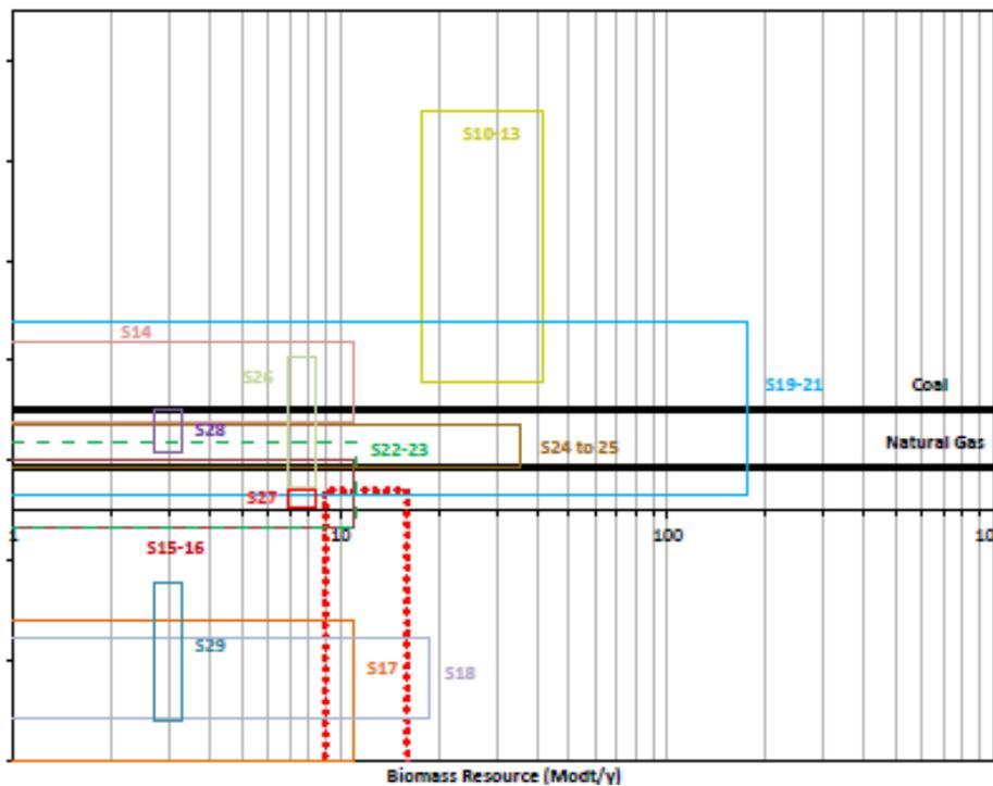
Figure 1: Global warming potentials for biomass power production from a range of different sources (coloured boxes represent ranges in emissions and available resources) compared to power production from coal and natural gas [Stephenson and MacKay]
