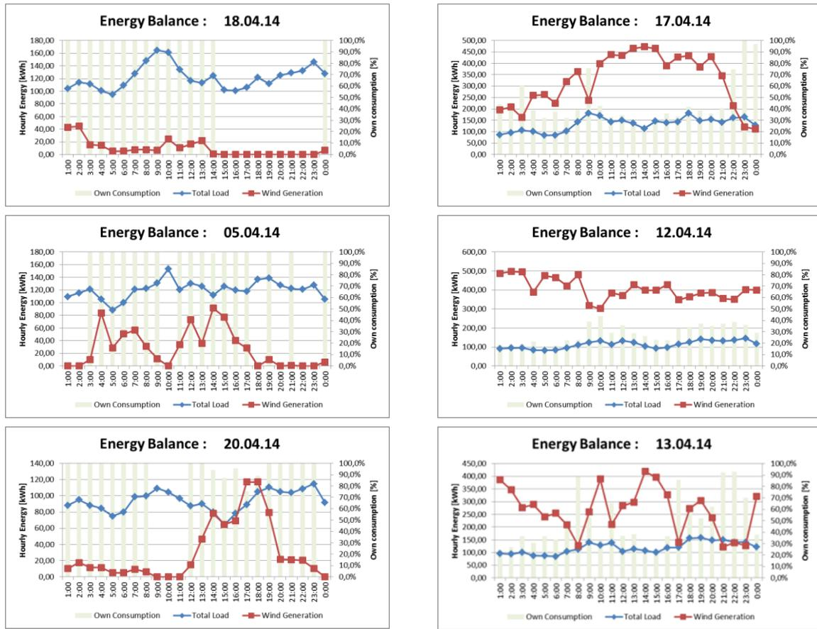
Figure 12: Wind generation, load and self-consumption for selected days in April 2014.
