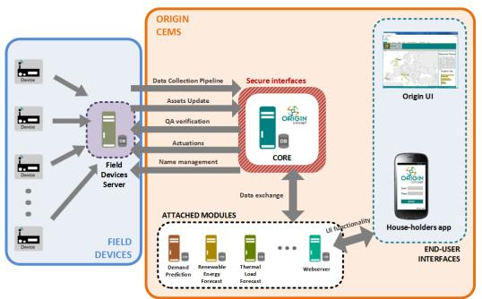
Figure 3.1 - ORIGIN platform high-level architecture
