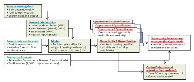
Figure 2.6: Flowchart for the thermal model predictive control algorithm
