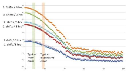
Figure 1.6: Modelling the outcomes of residential demand response scenarios as a function of forecast error, simulated based on Findhorn data. Vertical axis is utilisation of available wind energy, while horizontal axis is wind-speed forecast error. For scenarios refer to text.
