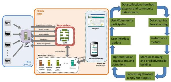
Figure 1.1: Characterising end-to-end operation (right) of the ORIGIN control architecture (left)
