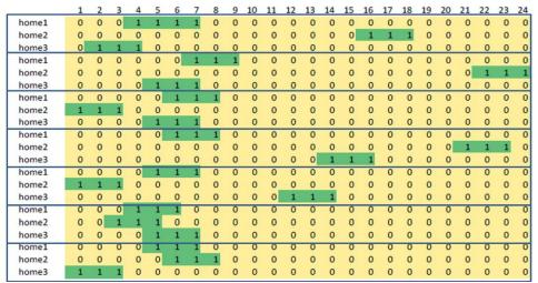
Figure 1.5: Actuations at three homes in Findhorn over a one-week period in November 2015; for example, on day 1, the hotwater system in home1 was automatically turned on at 04:00, and turned off at 07:00.
