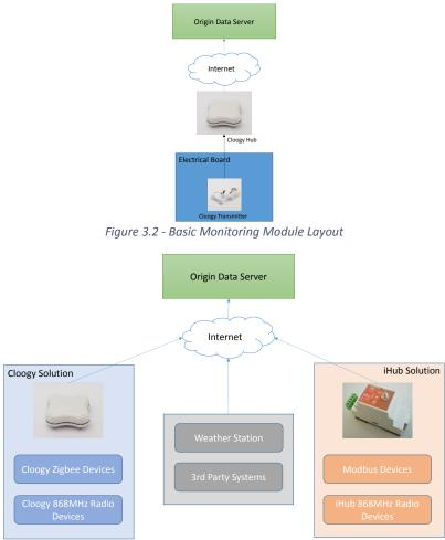
Figure 3.3 - Advanced Monitoring Module Layout
