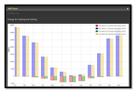
Figure 13: eKPI chart "energy" in nD Navigator for comparing different alternatives
