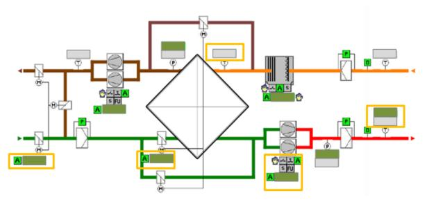
Figure 28: Key parameters – minimum data set for system performance monitoring
