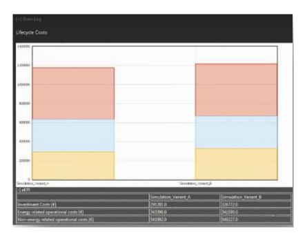
Figure 14: eKPI chart "life cycle costs" in nD Navigator for comparing different alternatives
