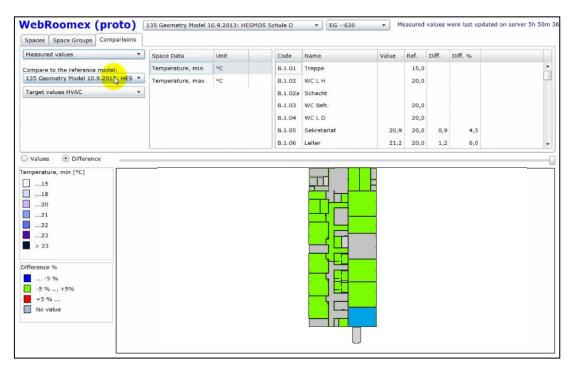
Figure 33: Comparison of measured data with targets on WebRoomEX interface
