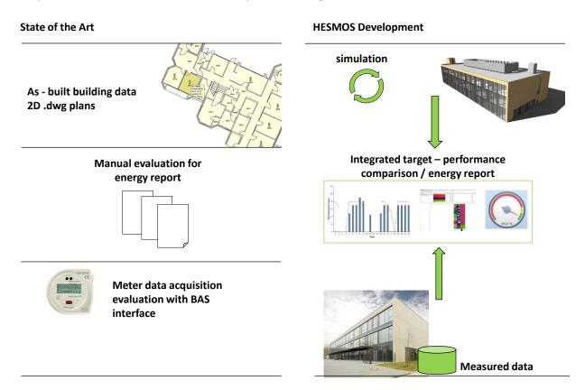
Figure 25: Comparison of state of the art and HESMOS developments during operation phase
