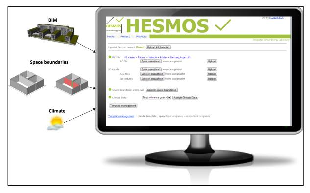
Figure 5: HESMOS platform – upload of IFC and conversion for simulations
