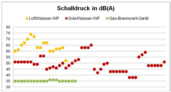
Figure 4.3: Comparative noise emissions of different heat generators
