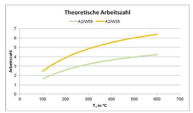
Figure 2-1: Theoretically possible EERs for gas heat pumps as a function of heat source temperature
