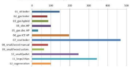
NOx emission NEW 2010, mg per kWh thermal output
