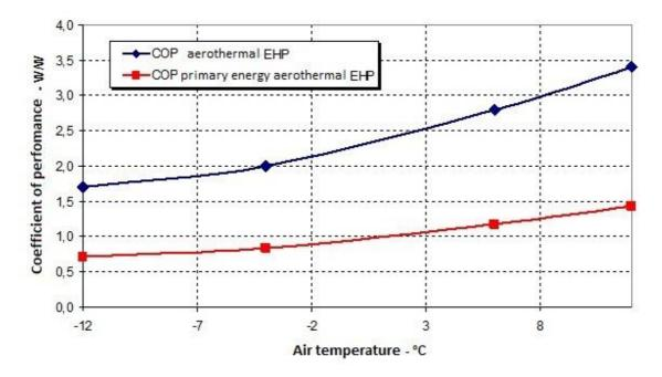
Thermal performance of an aero thermal EHP (outlet  $50^{\circ}$  C); conversion factor = 2.5 for primary energy calculation.
