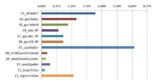
CO2 emissions NEW 2010, kg per kWh thermal output
