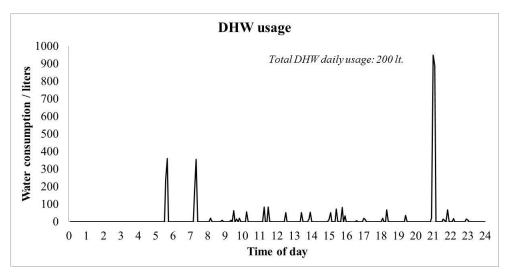
Figure A-2. Example of the DHW usage profile time-averaged at 5 minutes in a flat (FC+COGEN-SIM project, 2007, IEA Annex 42).
