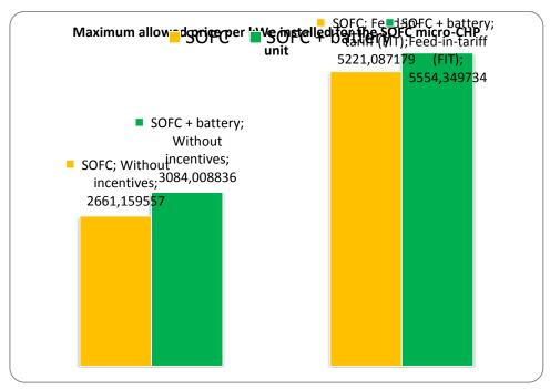
Figure 2-15. Allowed price per kWe of the SOFC generator that enables a return-of-the-investment within 5 years for the residential end-user (large family household).
