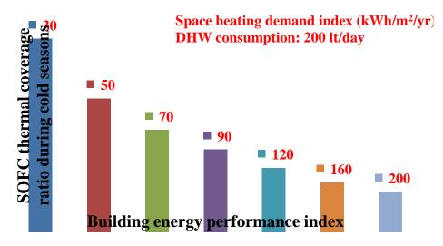
Figure A-3: Simulation of the share of the overall thermal demand provided by the SOFC to the 'average' household according to its energy performance index.
