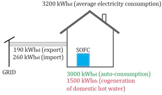
Figure 4-2: Energy flows in the micro-CHP unit.
