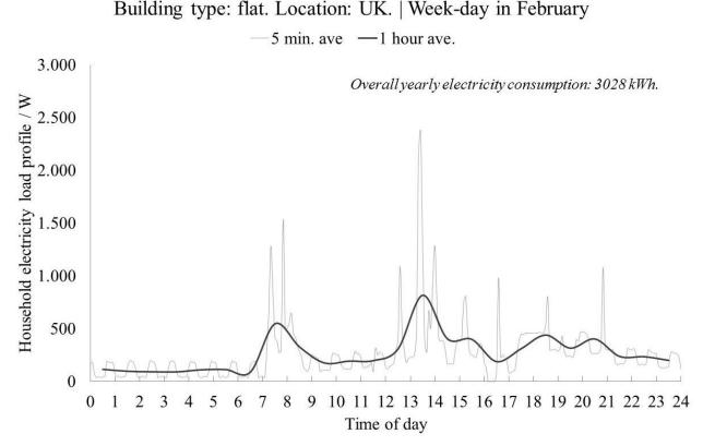
Figure A-1. Example of the electric load profile time-averaged at 5 minutes and 1 hour, respectively, in a flat (FC+COGEN-SIM project, 2007, IEA Annex 42).
