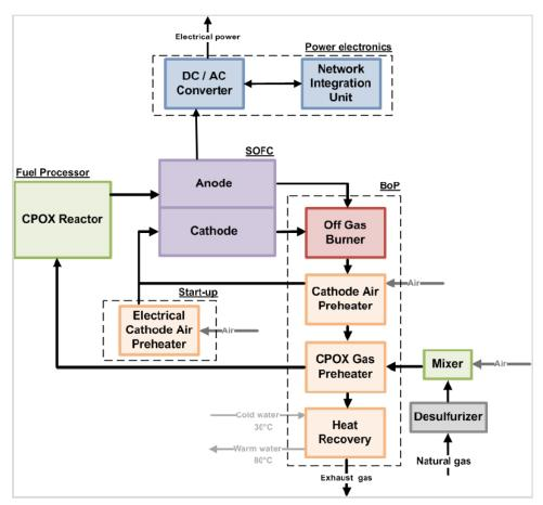
Figure C-1. Schematic representation of the FC-district μ-CHP layout with C-POX fuel processor [7].
