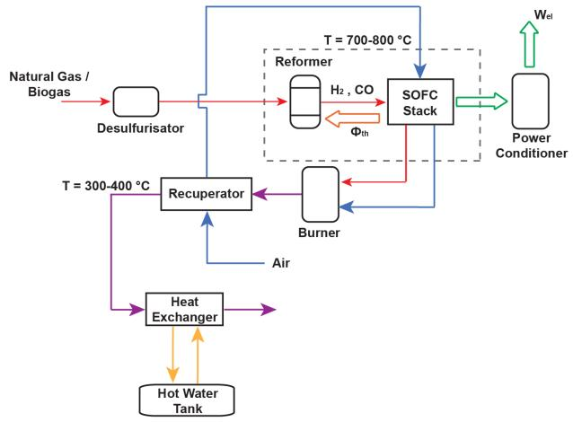
Figure C-2. Schematic representation of the FC-district µ-CHP layout with steam-reforming fuel processor.
